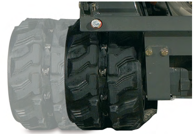
Hydraulically adjust the track width for added stability and traction.
