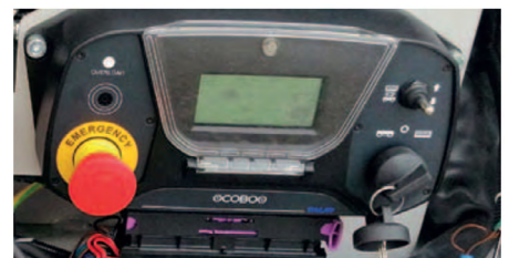
New ground control panel with integrated display for data retrieval and troubleshooting.
