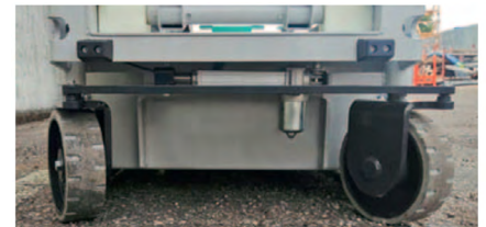
Front electric steering enabling maximum precision of movements.
