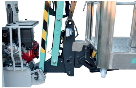
Compact jib assembly hosting both the load sensor and basket rotation system.
